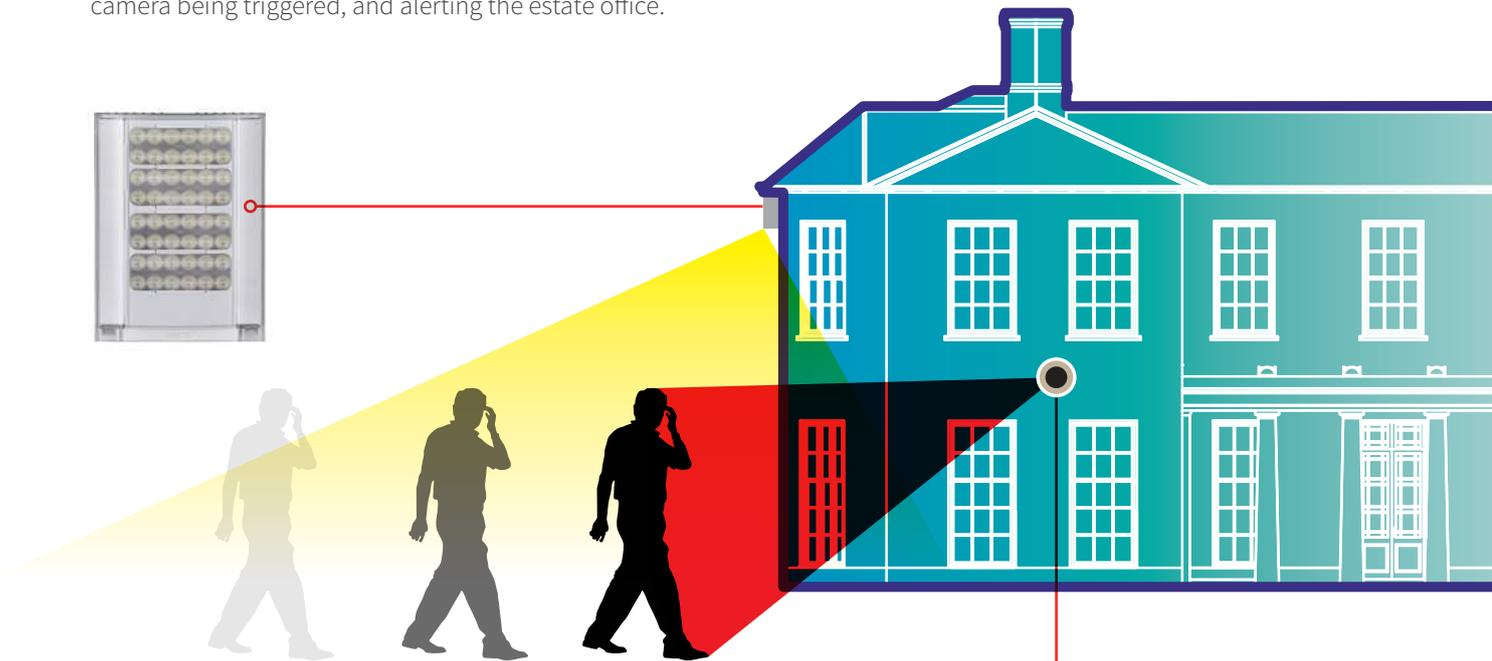
As well as being a deterrent, the combination of security lighting with PTZ cameras improved the quality of the footage, captured on the network video recorder, for a number of static dome CCTV cameras allowing the intruders to be identified.
